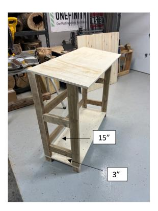
Using pocket hole screws, insert support 2x4's in the sides and at the rear. Install at 3" height and at 15" height.
