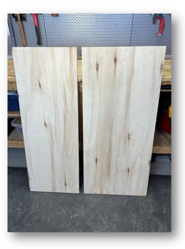
\*These are the bottom and the roof sheets. The larger one is the roof to provide an overhang for water to drip away from the wood pile.
