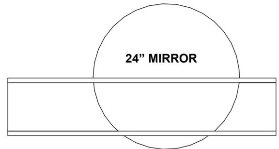
3. Assemble with pocket holes and screws. The shelf unit can be attached to the wall by screwing through the back panel in the area that the mirror will cover.
