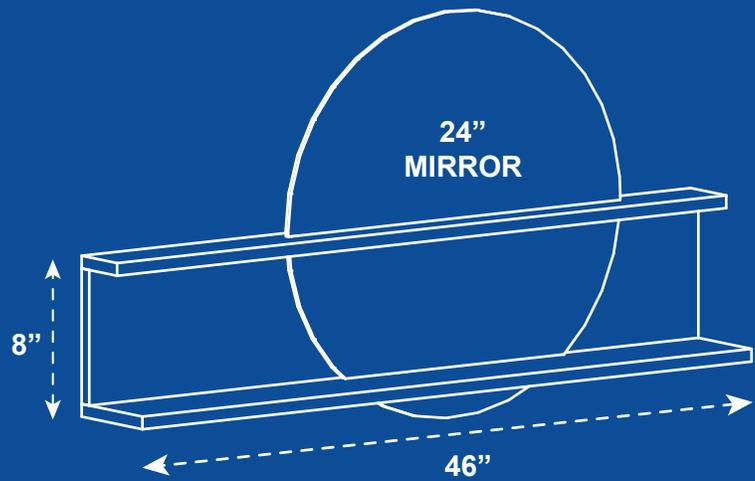
1. Cut three pieces of plywood. These are the sizes i used but this design idea can be adapted in all dimensions.
