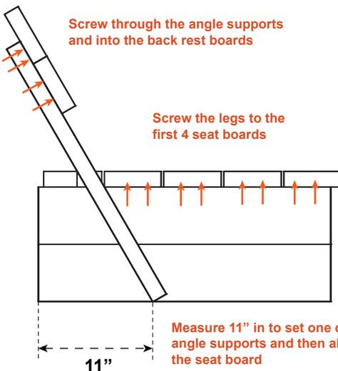
Use pocket holes to screw angle supports to inside of leg panels
