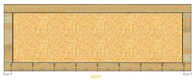
Create pocket holes that are 9" apart along the bottom of the panel.
