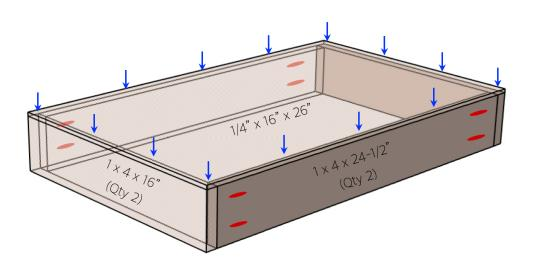
Drill pocket holes and assemble drawer box with wood glue, 1-1/4" pocket screws, and 1-1/4" brad nails
