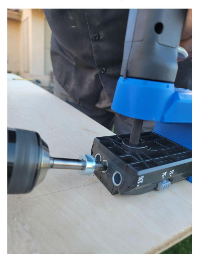
**Step 4**: Attach the 1  $\times$  3" to the plywood topper. Start with the ends - Apply glue to the edge of the plywood prior to attachment. Using 1" Kreg screw, attach the end to the top. Repeat the same step on the other end.
