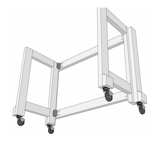
Attach the 2 1/2" locking casters to the back stationary legs of the bench and the fronts of the folding panels.
