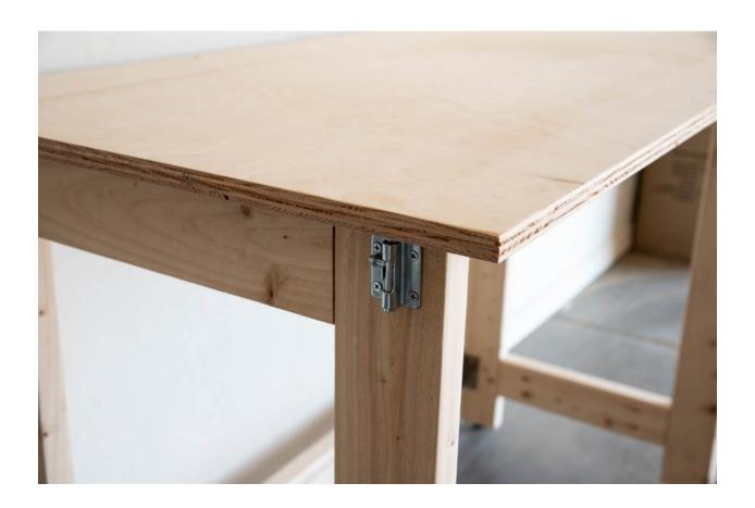
Install barrel bolt latches on the front legs (latches only, not the catch). The latches should be installed approximately 1/4" down from the top of the legs. Set the bolt against the top of the plywood and trace around it with a pencil. Move the leg out of the way and drill a 5/16" hole where the mark was traced. The bolt will fit into the hole and then turn and lock in place to secure the leg. Repeat this step on the other side of the table.
