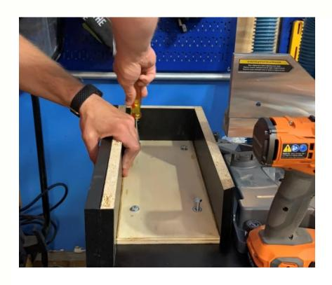
Next, we will add the plywood panel that will attach to the side of the melamine vertical of the deck. This panel is flush with the bottom of the bench top and about ¾" lower than the black melamine sides. This piece will dictate the height of the wings and hold the hinges. Again, secure using glue and brad nails. The hinge screws were 2" long and went into all three pieces for a nice solid engagement.
