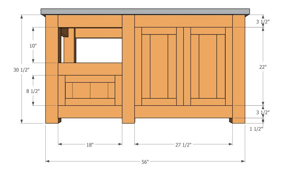
View of Front Assembly From Rear (Showing Leg Grooves on Front Legs)
