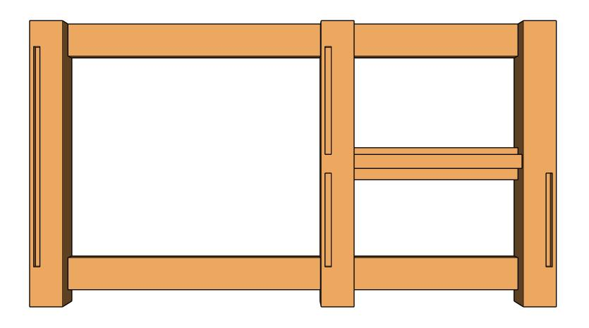
View of Rear Assembly From Front (Showing Leg Grooves on Rear Legs)
