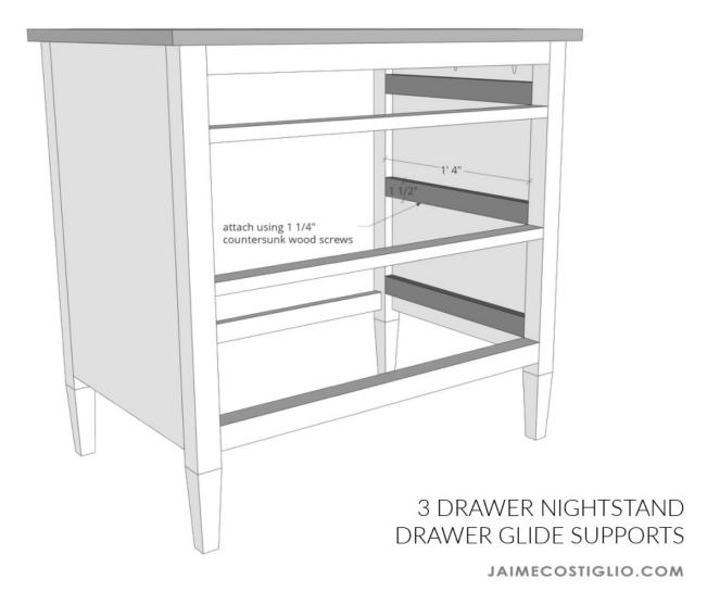
Before installing drawer glides attach supports to interior side panels using wood glue and 1  $\frac{1}{4}$ " countersunk wood screws.
