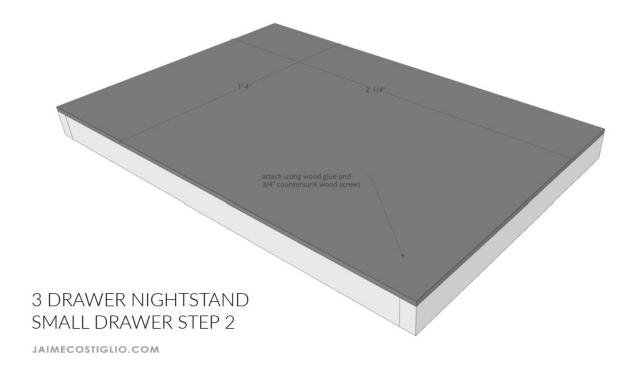
Step 2: Attach drawer bottom to box using wood glue and 3/4" countersunk wood screws.
