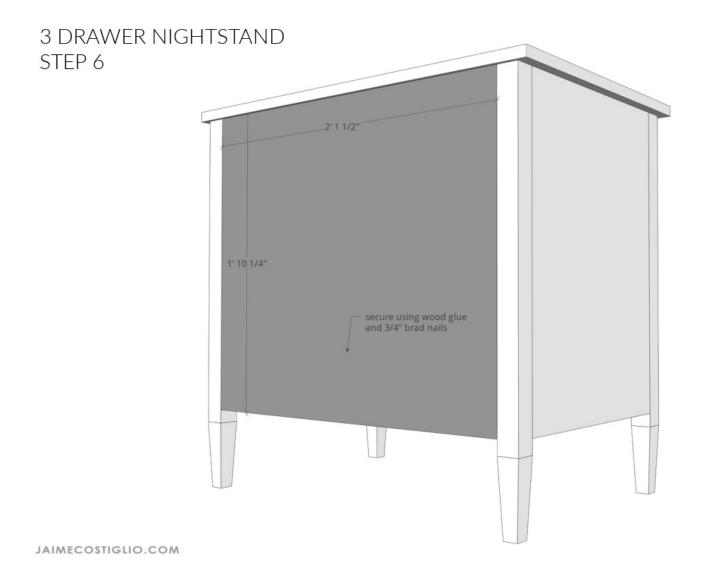
Step 6: Attach backing to cross supports using wood glue and 3/4" brad nails.
