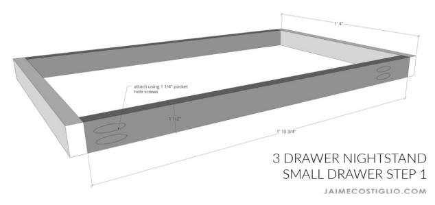
Step 1: Attach long sides to short sides using wood glue and 1 1/4" pocket hole screws.
