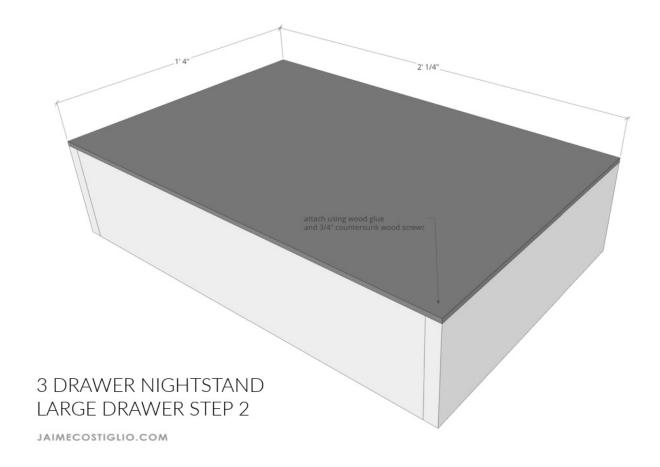
**Step 2:** Attach drawer bottom to box using wood glue and 3/4" countersunk wood screws.
