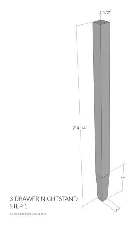
**Step 1:** If desired use a tapering jig to make bottom portion of legs tapered.
