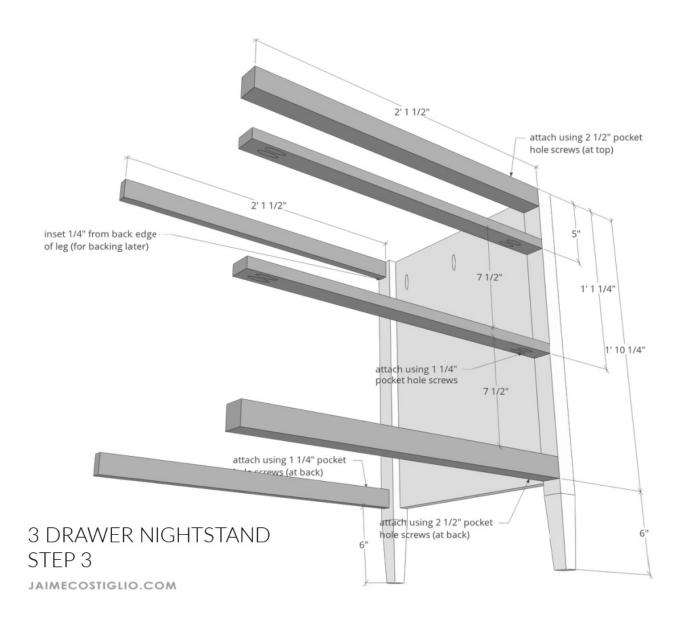
**Step 3:** Attach cross supports to side panel. Use wood glue and corresponding pocket hole screws. Keep pocket holes at back, top or underside when possible.
