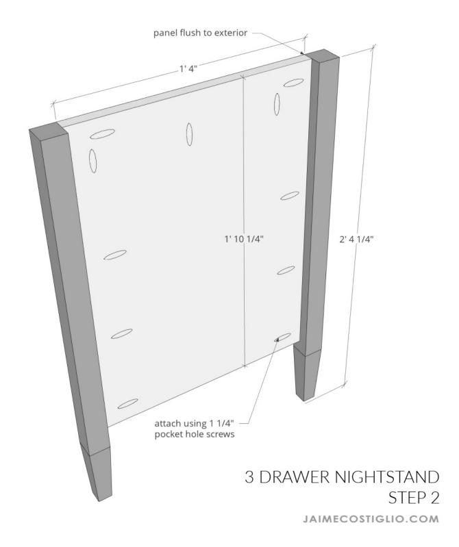
**Step 2:** Attach legs to side panels using 1 ½" pocket hole screws. Keep side panel flush to leg at exterior. Make 2.
