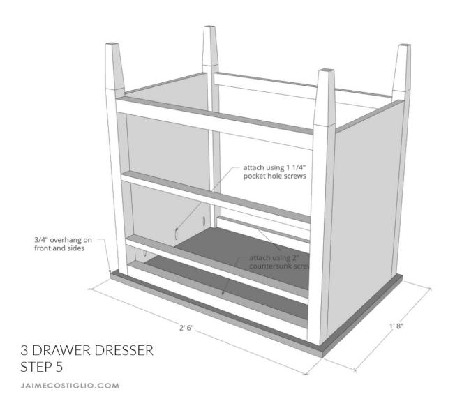
**Step 5:** Attach top to body using 1  $\frac{1}{4}$ " pocket hole screws. Keep  $\frac{3}{4}$ " overhang at front and sides. Secure front and back cross supports to top using 2" countersunk wood screws.
