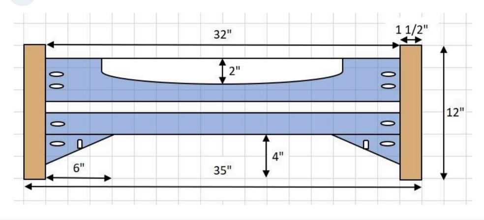
**Pocket holes side** Pocket holes placement for the side boards and bottom braces.
