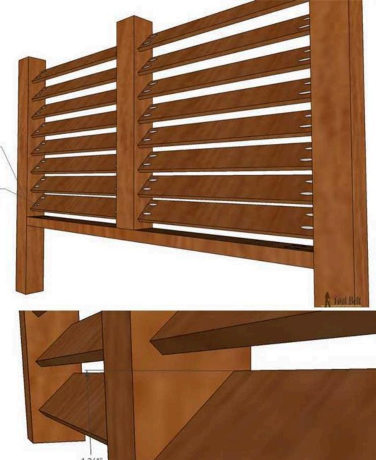
Start from the bottom – and line up louver slat corners with marks and secure with 1" pocket hole screws.
