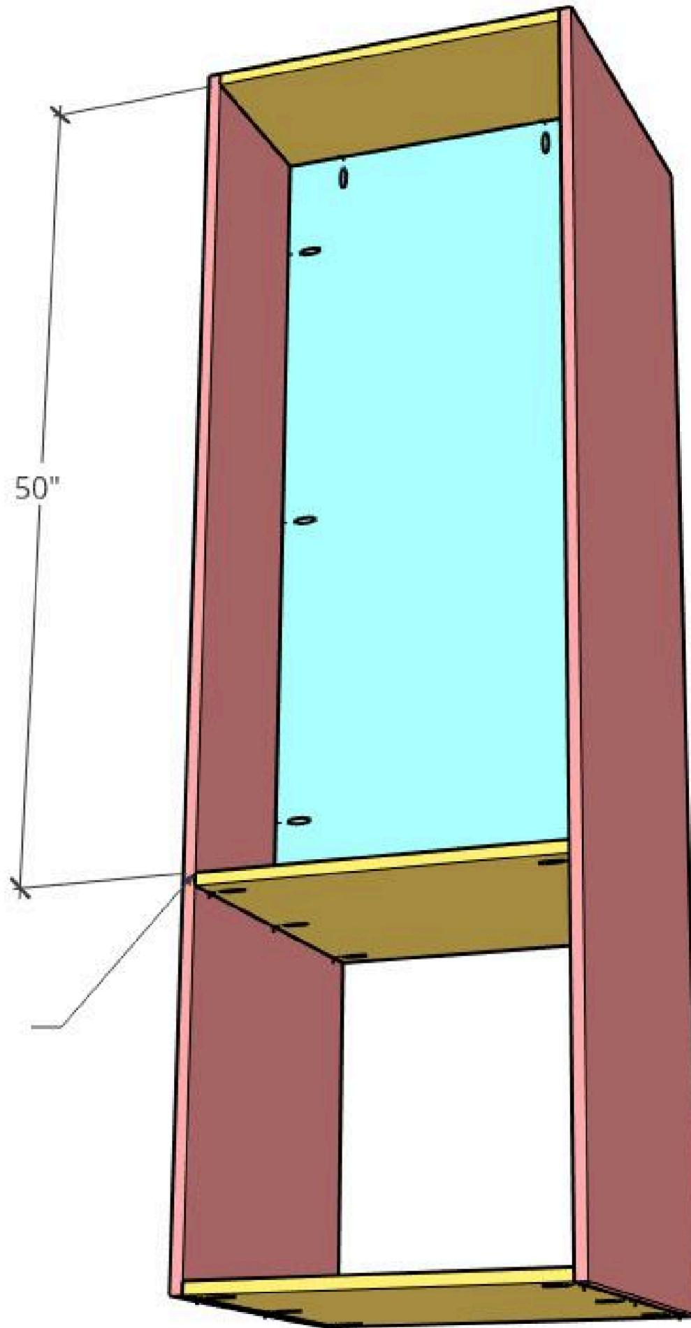
Attach shelf to sides with 3/4" pocket holes and 1 1/4" pocket hole screws
