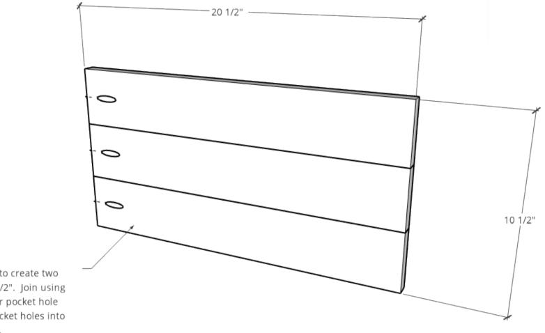
Join 1x4s like shown to create two panels 10 1/2" x 20 1/2". Join using wood glue, dowels, or pocket hole joinery. Drill 3/4" pocket holes into ONE END like shown.
