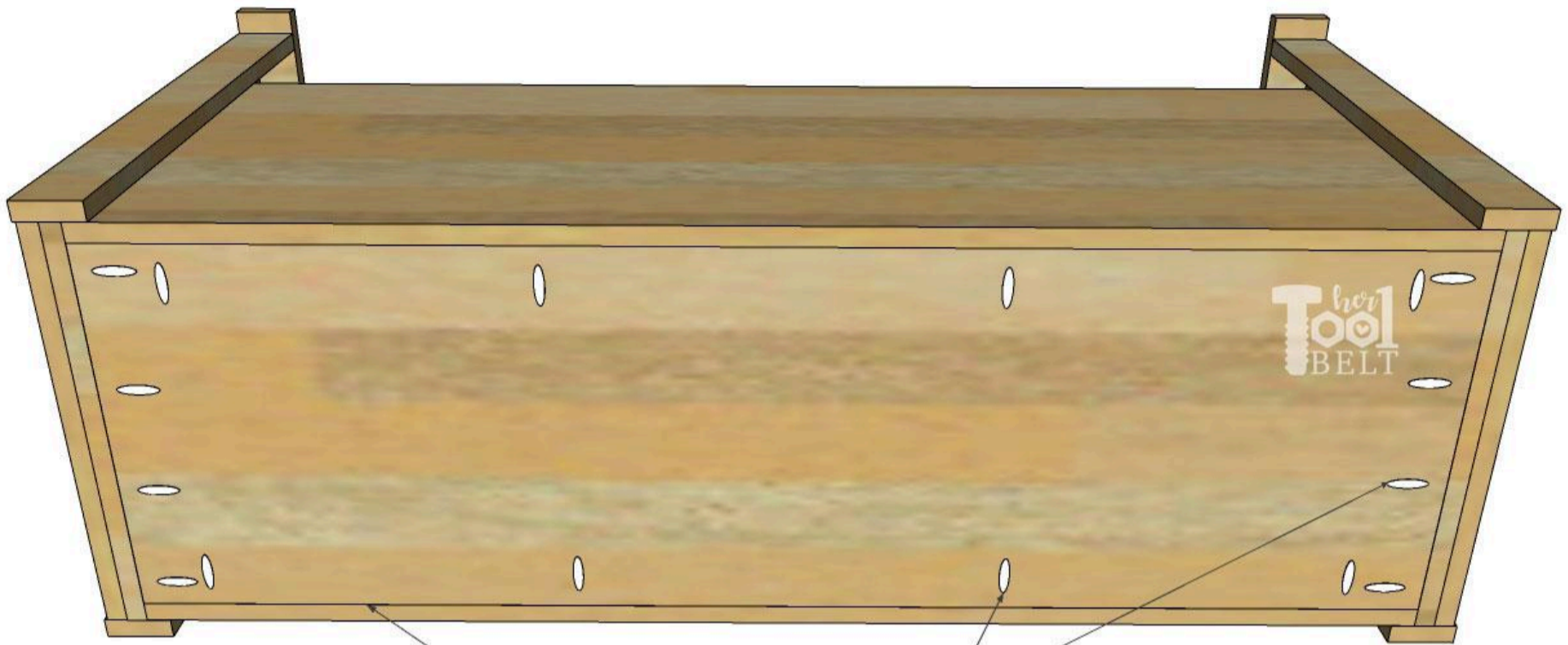
Use wood glue and 1 1/4" pocket hole screws to attach box bottom to box front/sides/back.
