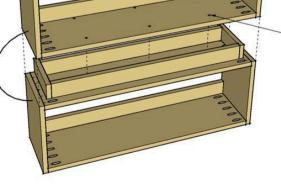
Drill holes in upper shelf of middle assembly. See the illustration in Step #1 for hole locations.
