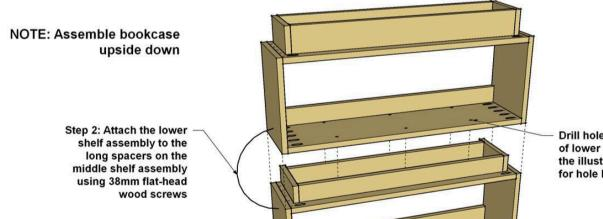
Drill holes in upper shelf of lower assembly. See the illustration in Step #1 for hole locations.
