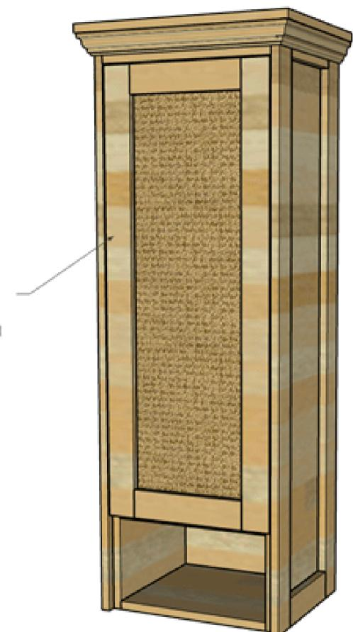
Install door using full overlay concealed hinges for frameless cabinets leaving 1/8" gap around top and sides
