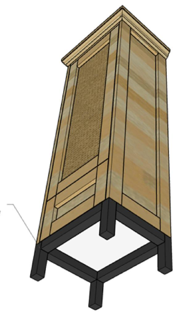
Use 2" wood screws to secure base to bottom of cabinet
