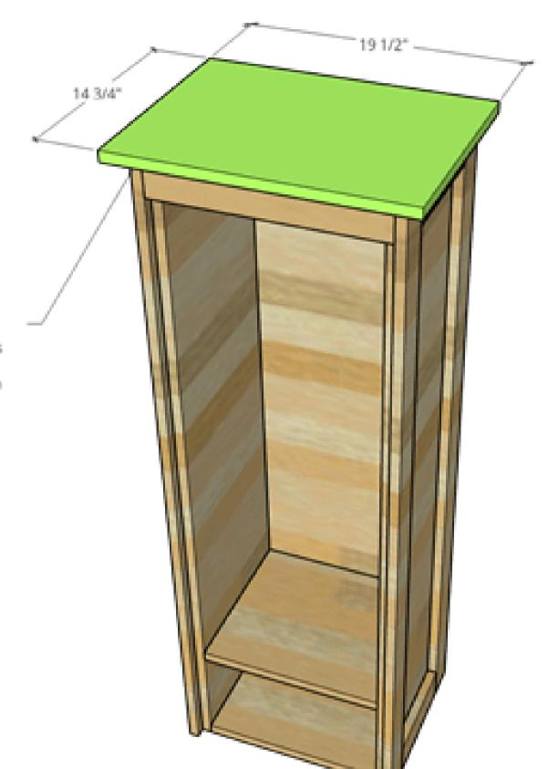
Screw 3/4" plywood top onto cabinet using 1 1/4" wood screws through top supports. Install flush to back side and with 1 1/4" overhang on each side.
