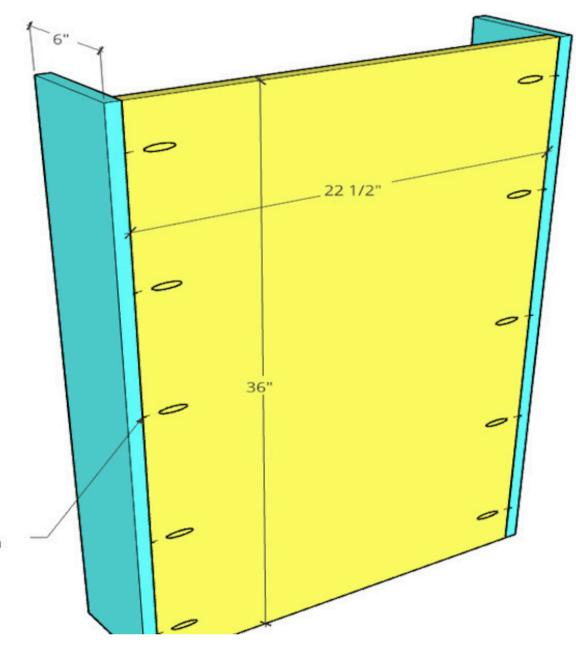
Assemble back panel between side panels using 3/4" pocket holes and 1 1/4" pocket hole screws
