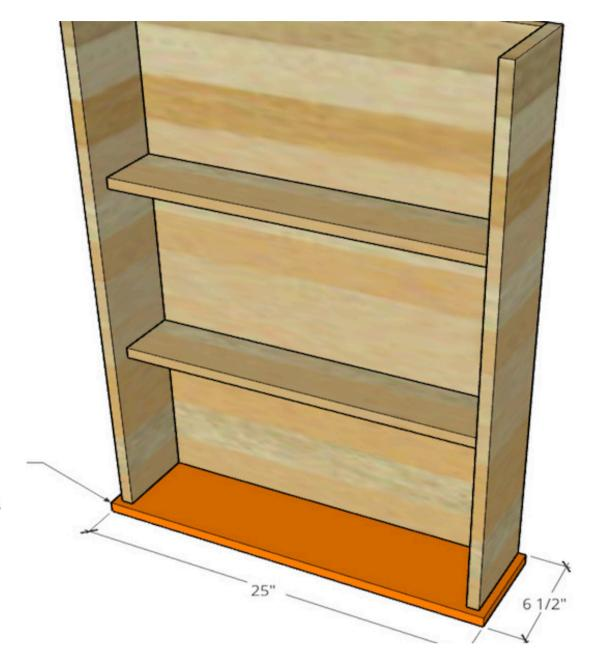
Use 1 1/4" wood screws through bottom panel up into sides/back panel to secure. Leave 1/2" overhang on sides and install so that it's flush across the back
