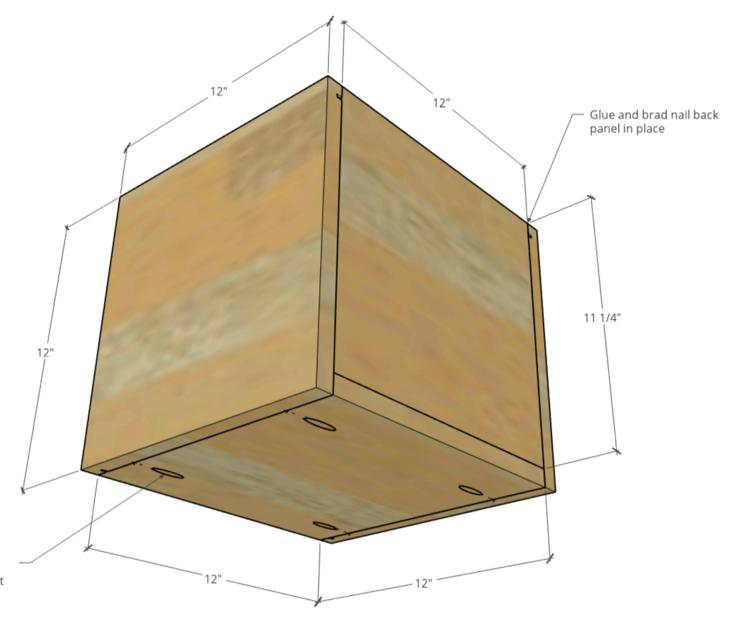
Assemble bottom between side panels using 3/4" pocket holes and 1 1/4" pocket hole screws
