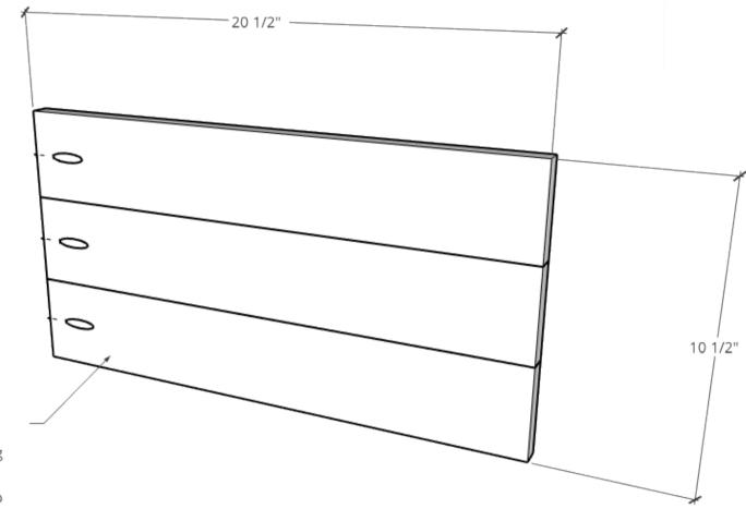
Join 1x4s like shown to create two panels 10 1/2" x 20 1/2". Join using wood glue, dowels, or pocket hole joinery. Drill 3/4" pocket holes into ONE END like shown.
