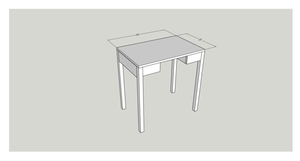
Notch out the bottom of the desk with a jigsaw, then attach using 1 1/4" pocket screws and wood glue.
