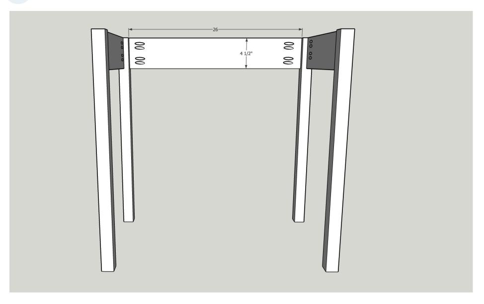
Attach front dividers using 1 1/4" pocket screws and wood glue.
